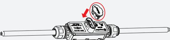
*Note: Under the circumstance that need to remove the inverter AC cable from 3P-AC bus connector, please use the 3P-AC connector unlock tool and insert the tool into the side of AC port to remove.*
